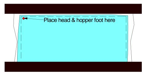
Move Statler head to the upperleft corner of the fabric such that when the pattern sews out the top and left edge will be on the fabric.
