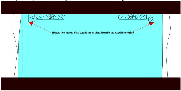
Click measure, measure from end of the outside line on the left to the end of the outside line on the right. Highlight "glcq pass2 w crown" pattern, click repeat pattern. Position head at end of outside line on left. Change the pattern width (freeze on) to what you measured or transfer in the length and then transfer the angle into Square Up Quilt Angle.
